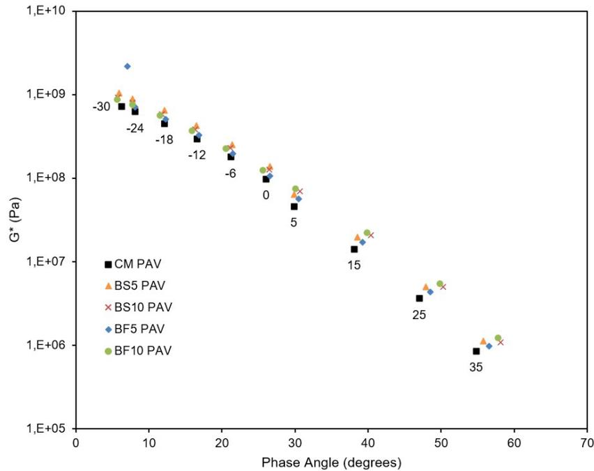
Figure 5. Black Space Diagram at 10.9 rad/s at varying temperatures in °C.
