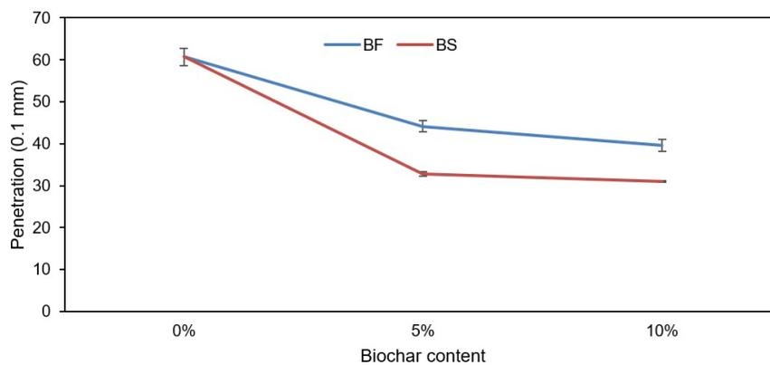
Figure 2. Penetration at 25°C.
