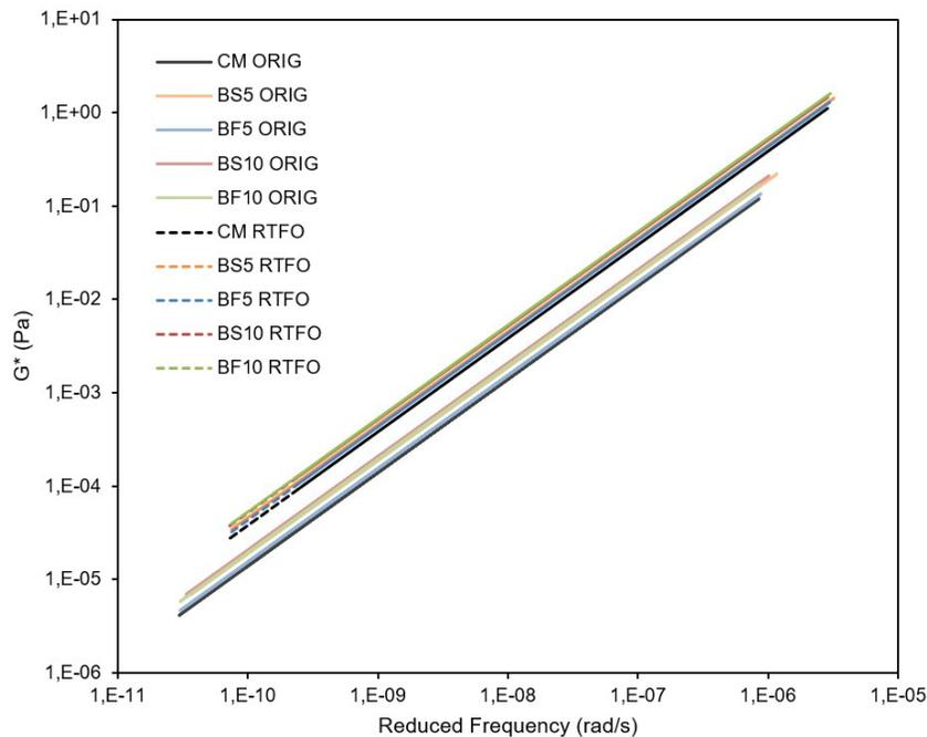
Figure 6. Master Curves at a reference temperature of 58 °C before and after RTFO.
