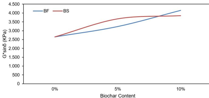
Figure 4. Superpave Fatigue Parameter of PAV residue at 25°C and 10.9 rad/s.
