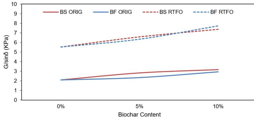
Figure 3. Superpave Rutting Parameter at 55°C and 10.9 rad/s.
