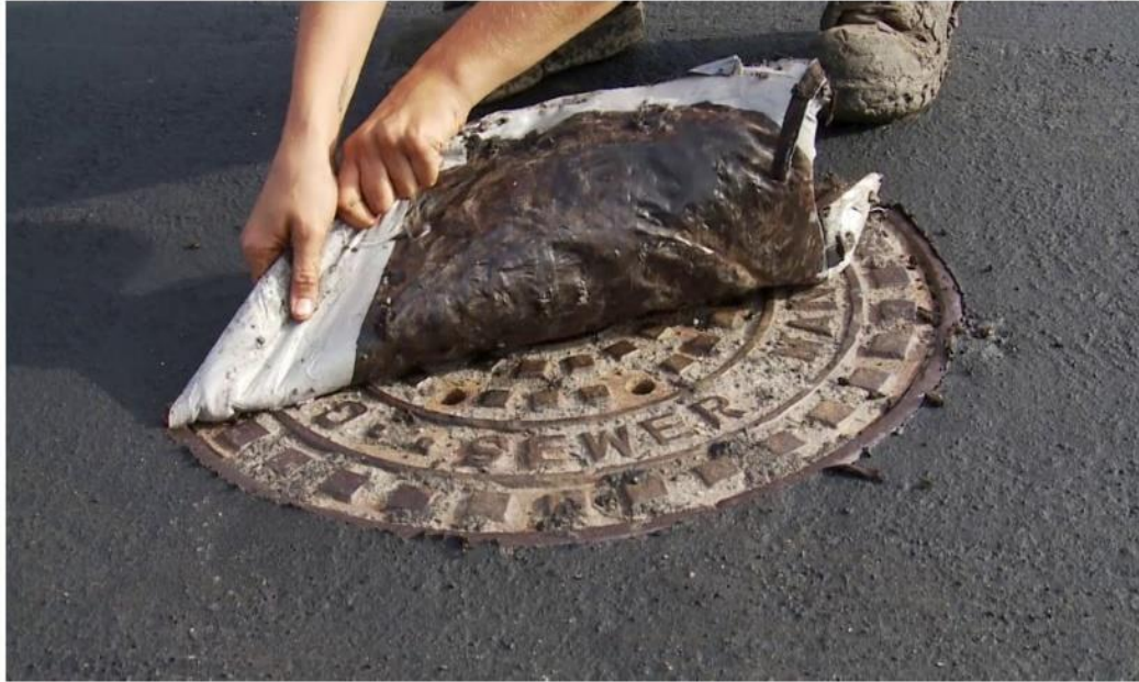
Figure 1. Slurry mix sample collected using plastic sheet placed over utility cover.
