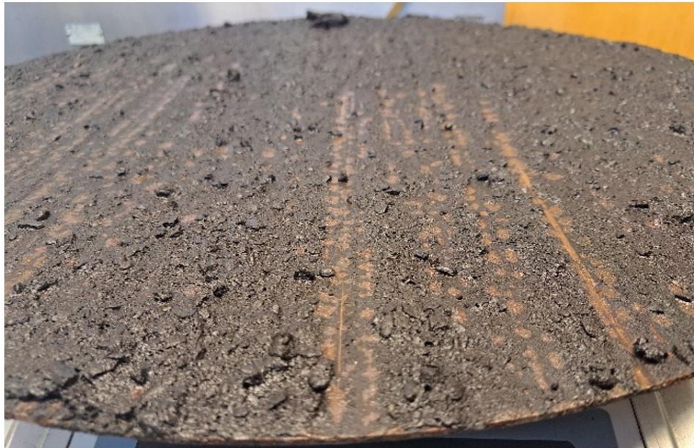
Figure 2. Slurry mix sample collected using aluminum plate placed over utility cover.
