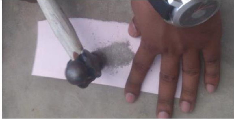
Figure 6. XRD sample hammered down to the required size
