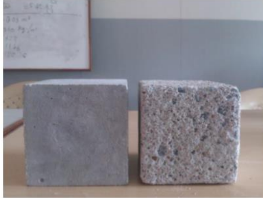
Figure 4. Specimens before and after acid attack test
