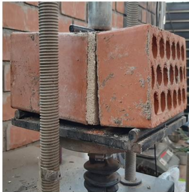
Figure 5. Flexural bond strength of prisms. (Source: Author).
