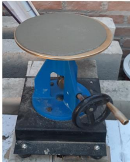
Figure 1. Mortar flow test. (Source: Author).
