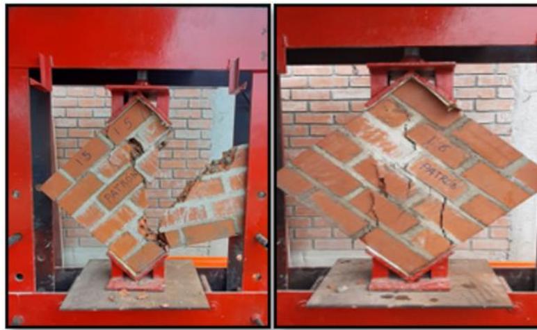
Figure 6. Elaboration of walls for diagonal compression test. (Source: Author).
