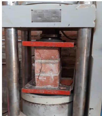
Figure 4. Compressive strength in masonry prisms ( f_m ). (Source: Author).
