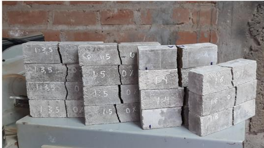
Figure 3. 40mm x 40mm x 160 mm specimens tested in flexure. (Source: Author).
