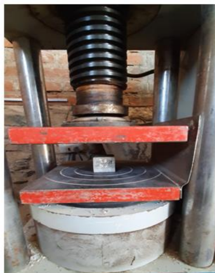
Figure 2. Compressive strength of cubic specimens of 50 mm side. (Source: Author).
