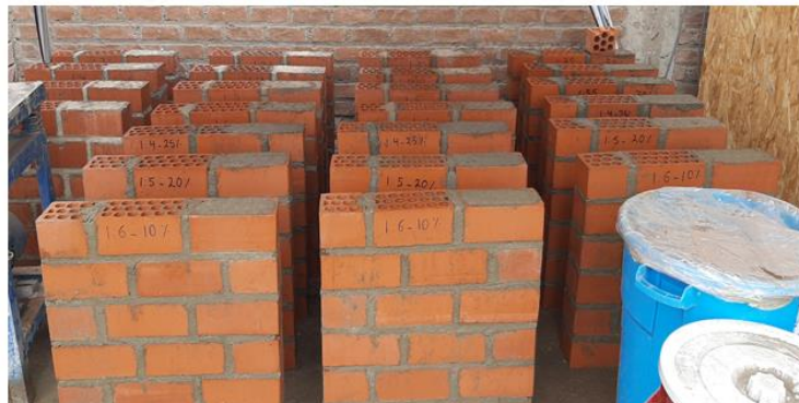
Figure 6. Elaboration of walls for diagonal compression test. (Source: Author).
