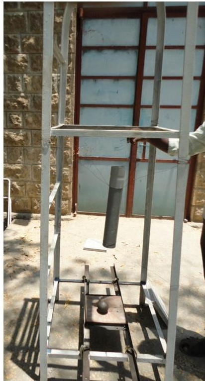
Figure 8. Flexure test setup
