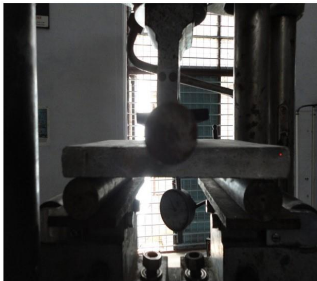
Figure 7. Flexure test setup
