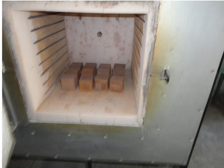
Figure 1. Fire exposure of Cube specimens
