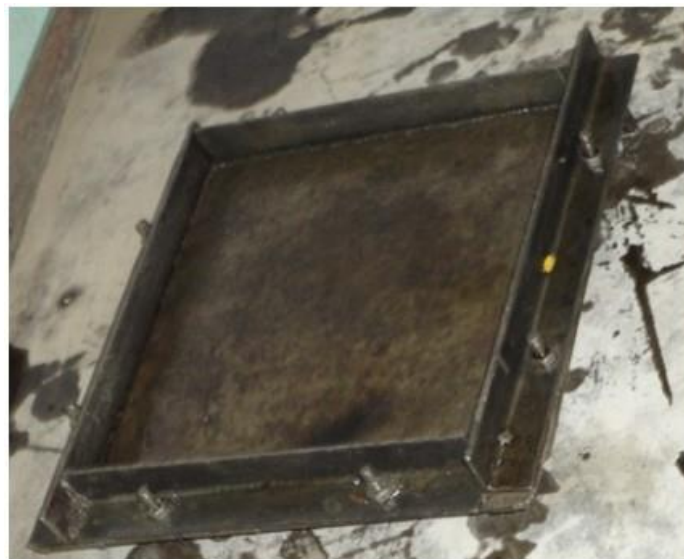
Figure 2. Mould used for casting
