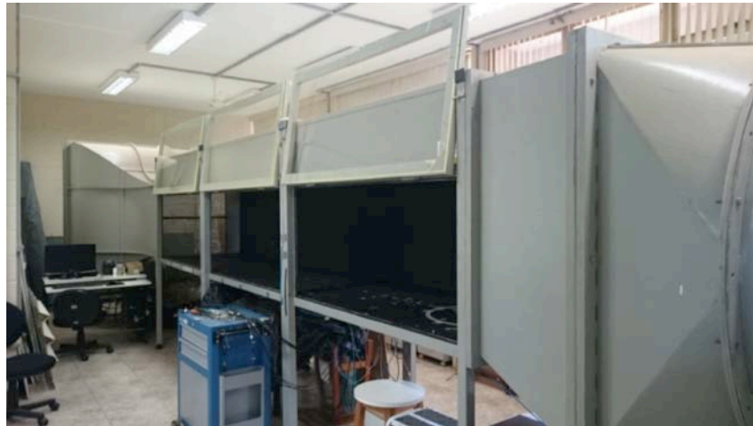
Figure 1. View of the wind-tunnel. On the left, the cone where the air comes in suctioned by the fan on the right.
